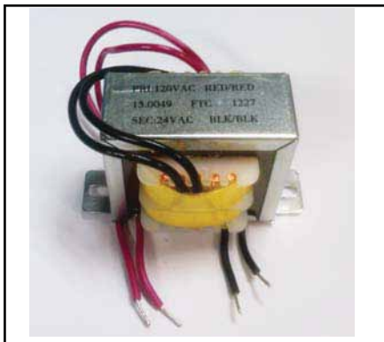
24VAC 24vAC TRANSFORMER
