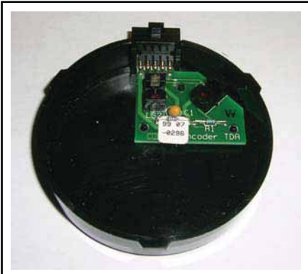
EEP.0001 ENCODER (WITHOUT DISK AND CABLE)
