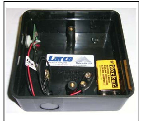
US800327 433MHz RADIO CONTROL TO CONVERT 4 1/2" ROUND HARDWIRE WALL SWITCH TO RADIO CONTROL
