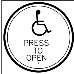
WALL SWITCH STAINLESS STEEL 4 1/2" DIAMETER ENGRAVED LOGO PRESS TO OPEN (HCPTO)
